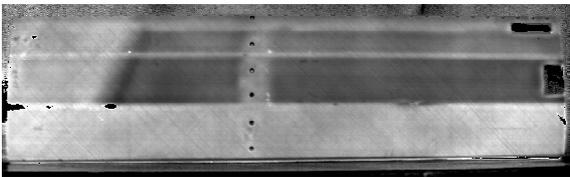
Fig. 3. Thickness image of a landing flap.
