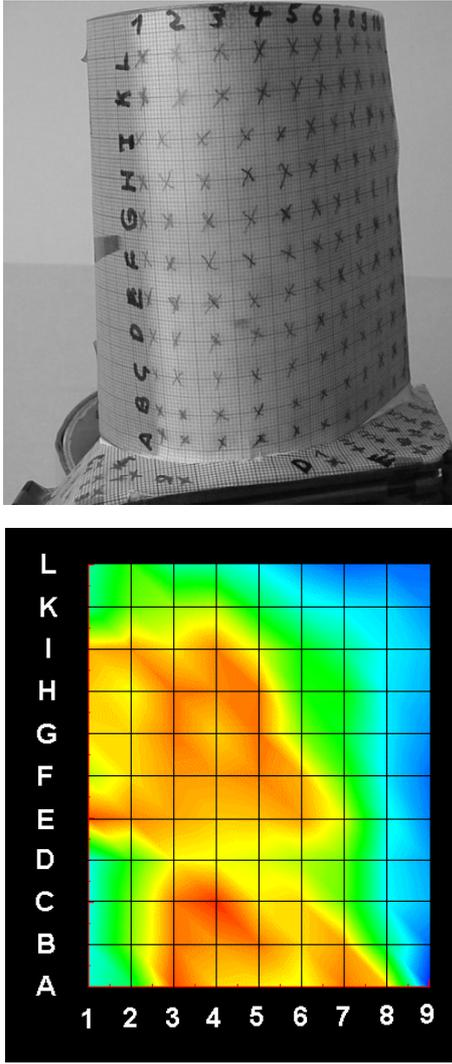
Fig. 1. Turbine blade with thermal barrier coating (top). Calibrated thickness image (bottom). Thick areas are marked red, thin areas blue.
