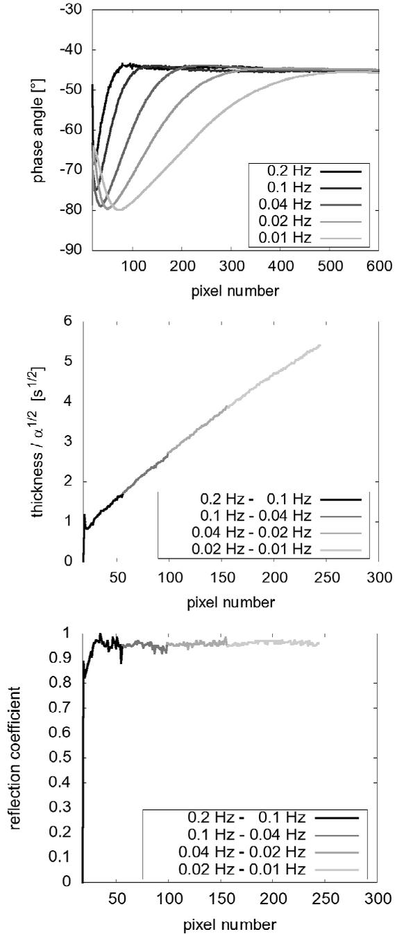
Fig. 2. Phase values along a polymer wedge for five different lockin frequencies (top). Calculated thickness (middle) and reflection coefficient curves (bottom).
